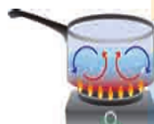
Gambar 3.11 Konveksi saat memasak air. Sumber: shutterstock.com/BlueRingMedia
